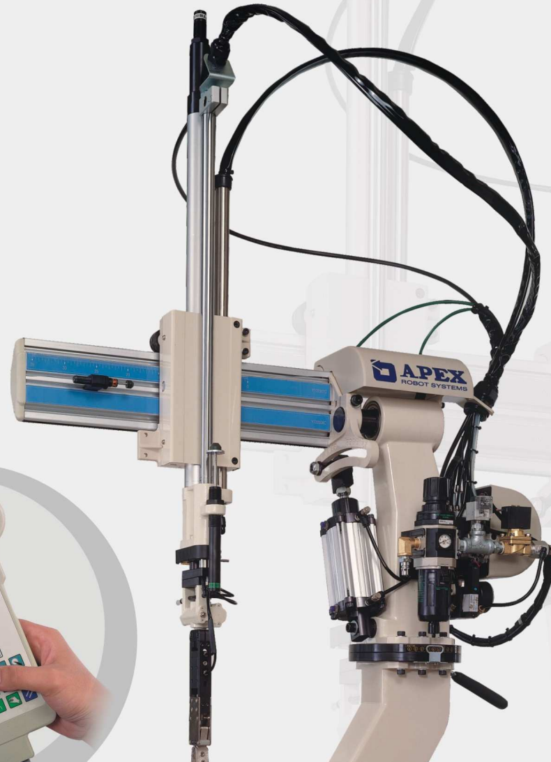
Simple base pivoting for ease of mold change.
