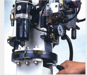
Simple base pivoting for ease of mold change.
